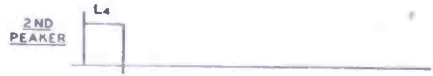
Fig. 7—Effect on a Square Wave with the peaker potentiometer open (second peaker).
